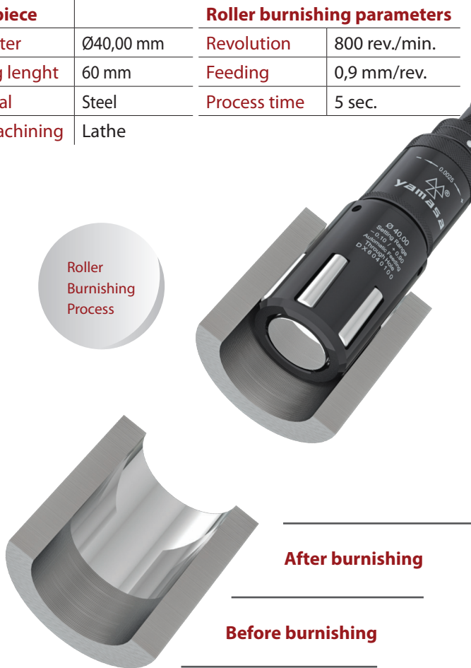
Figure 3 - Before and after roller burnishing surfaces
